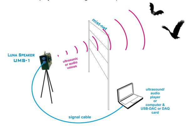
b) as an additional (second) audio or ultrasound active speaker connected to remote **LunaLure UMP-1** or **LunaLure UMP-2** device:
